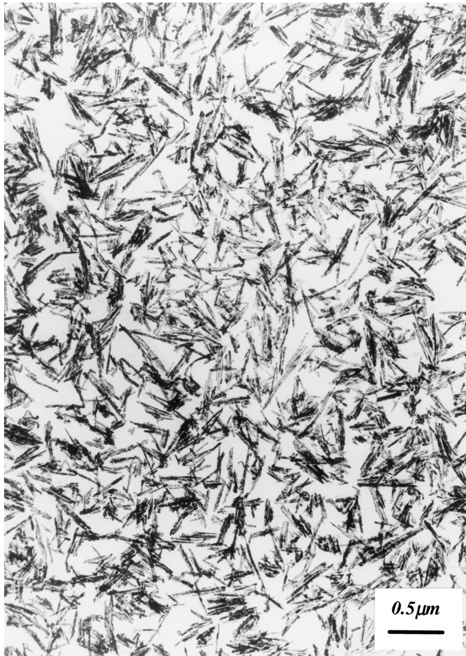
Figure 1 A typical transmission electron microscope image showing the morphology of very fine, acicular particles of \alpha -Fe prepared for 8 m/m video recording media. The particle is of a skeleton type and not the single crystal type. The image shows a mosaic structure consisting of grains with size in of order of 100 Å. The grain crystallographically belongs to the bcc phase and its shape is that of a rhombic dodecahedron. Sometimes, pores are included in the particles themselves. Furthermore, the particles easily form local aggregates which are called “multiple” or “bundle”.
